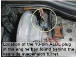
Figure 5 Location of 10-pin ALDL Test Plug in a Calibra.
